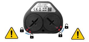
**CAUTION:** the battery surface may not be touched when installing the batteries into the sensor. Touching the battery surface will considerably <u>reduce the battery's lifetime</u> due to induced leakage current. Preassembled battery holders are available for easy battery replacement.
