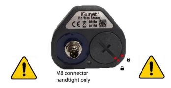
**CAUTION:** the battery surface may not be touched when installing the battery into the sensor. Touching the battery surface will considerably <u>reduce the battery's lifetime</u> due to induced leakage current. Preassembled battery holders are available for easy battery replacement.
